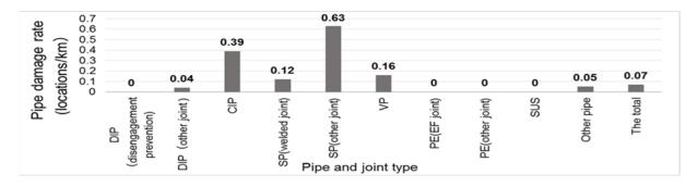
Figure 1. Pipe damage tare by pipe material in Kumamoto City
