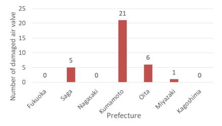
Figure 2. Number of damage to air valve in each prefecture
